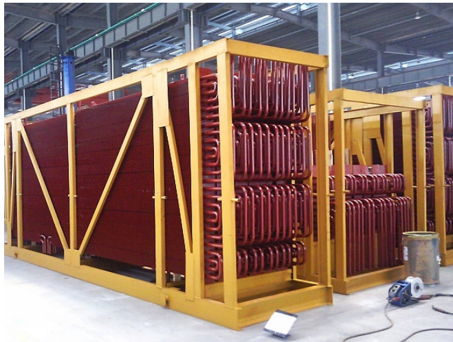
The first batch of Steel-H extended surface economisers for coal-fired power plants in India
