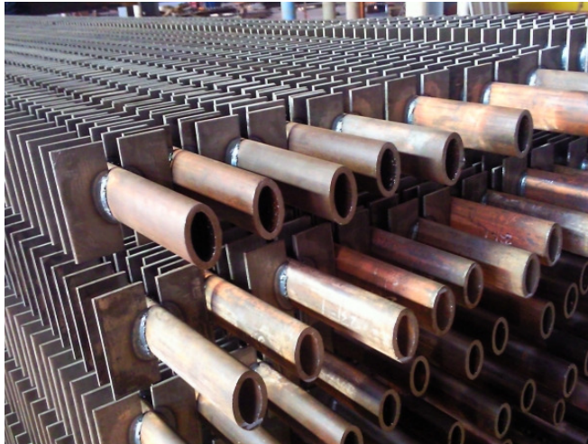
Oval shaped finned tubes for low temperature waste heat recovery
