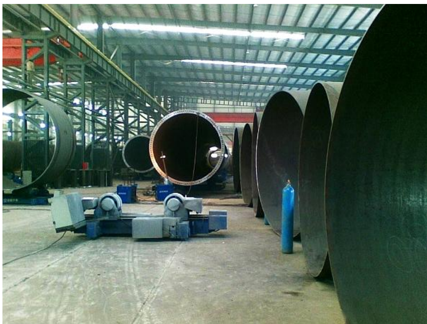
Production of steel towers for wind turbine inside the new plant
